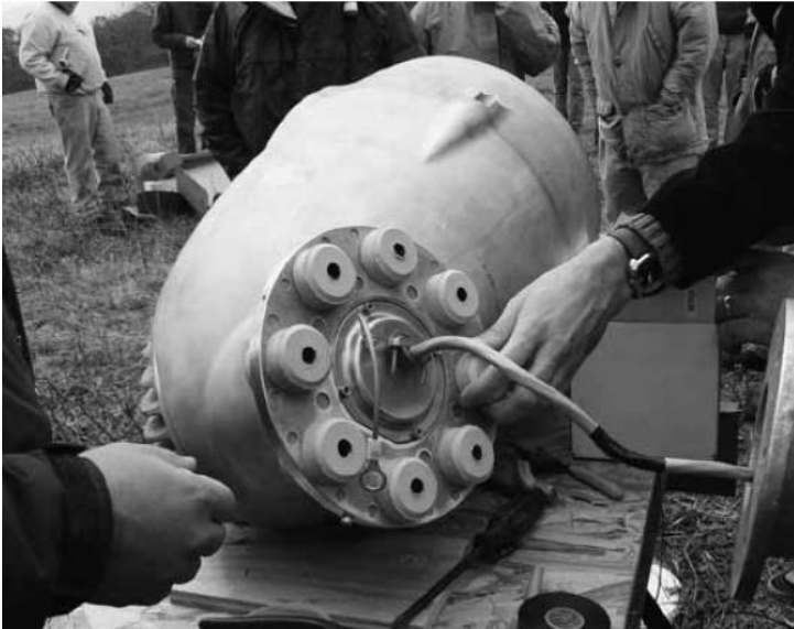
Figure 8 Placing vibration isolators
