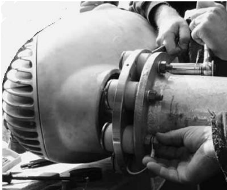
Figure 9 Grounding turbine to tower
