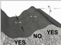
To maximize the performance of your wind turbine, it should be installed as far as possible from the obstruction and atop a tower higher point from this obstacle
